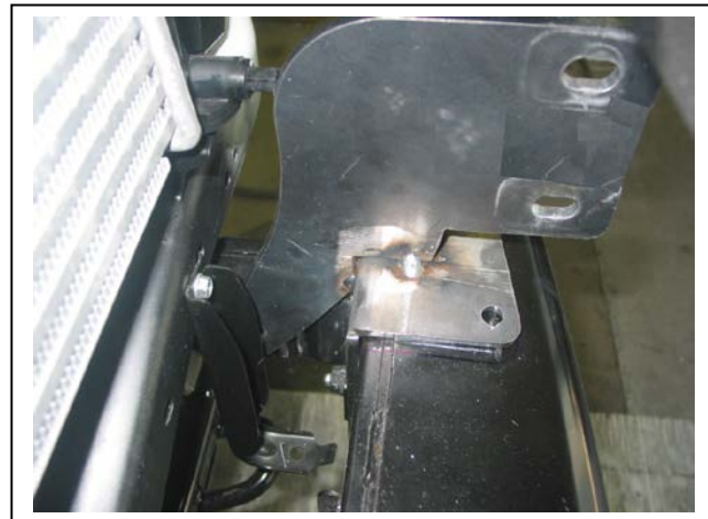
Figure 2: Passengers side mounting bracket in position
