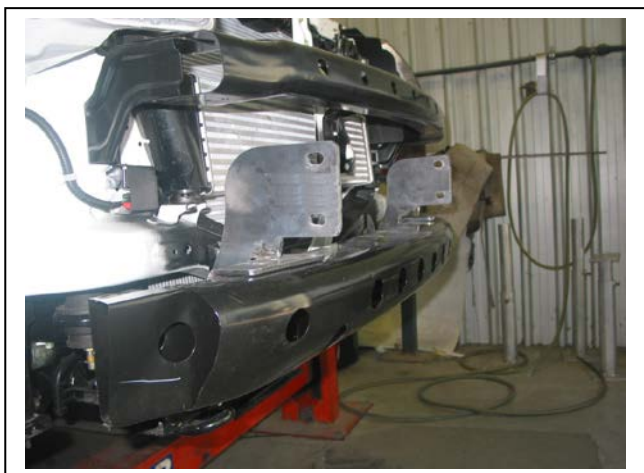
Figure 3: ECB steel mounting brackets fitted.
