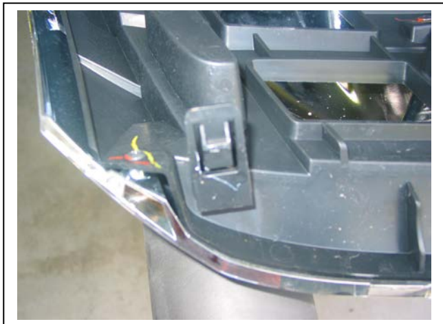
Figure 1: Lower outer clip on grille. Grille removed for photo.
