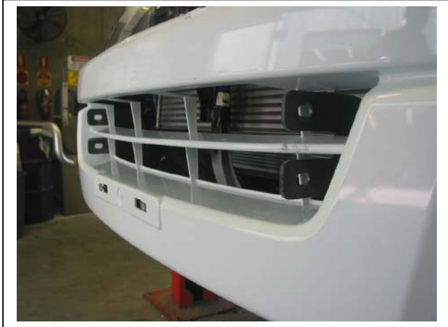
Figure 5: ECB steel mounts with bumper fitted. Isuzu Dmax shown
