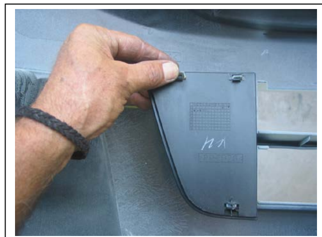
Figure 4: Remove passengers side blanking plate
